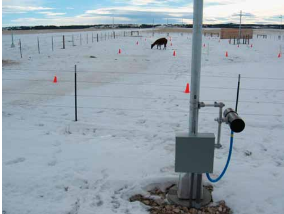
The test bed consists of animal detection systems, an enclosure for horses and llamas, infrared video cameras, and a remote office. The detection zones and detection lines were marked with cones to be able to record the position of the animals (Photo: Marcel Huijser, WTI/MSU).
